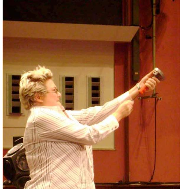
Figure 5: Blank Cartridge Firing Device
